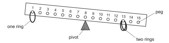
The wooden rod is uniform and all the rings are of equal mass. Two rings are hung on peg 13 and one on peg 1.
