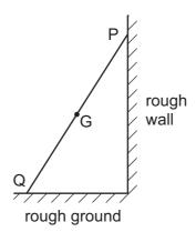
Its weight W acts through the centre of gravity G. Forces also act on the ladder at P and at Q. These forces are P and Q respectively.
